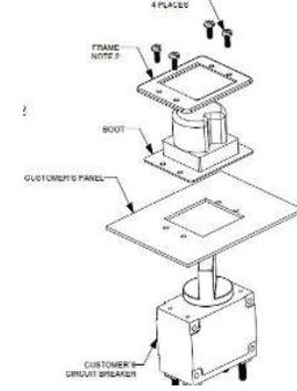
The boot needed to be able to hold up to the harsh weather conditions at sea as well as provide a reliable boot seal for a turn switch that had a 30° turn travel distance. In addition the design had to include both reliability as well as function to avoid interference with the breaker. **APM Hexseal** designed the turn switch breaker boot seal to every specification and included in the design
