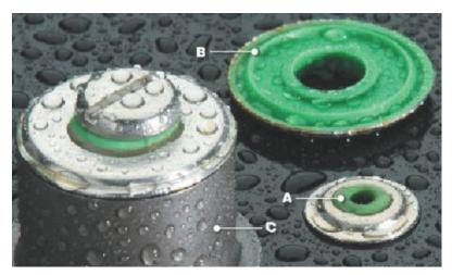
APM Hexseal SEELOC® self-sealing washers feature a silicone rubber section molded to a specially-formed stainless-steel washer. SEELOC pressure range exceeds 100 psi internal/external and is UL Recognized (UL Type 4X/6 enclosures) with an IP 66/68 water ingress rating. A variety of sealing materials and sizes, including metric, are available for specific applications. Temperature range of -160°F to +500°F (-106°C to 260°C).
