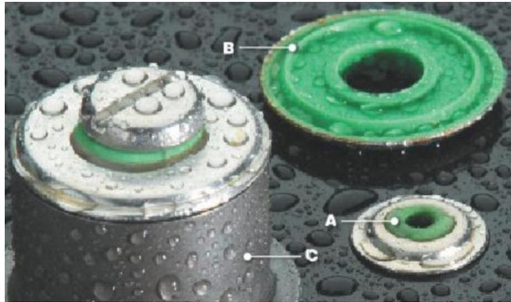
APM Hexseal [SEELOC® self-sealing washers](#) feature a silicone rubber section molded to a specially-formed stainless-steel washer. SEELOC pressure range exceeds 100 psi internal/external and is UL Recognized (UL Type 4X/6 enclosures) with an IP 66/68 water ingress rating. A variety of sealing materials and sizes, including metric, are available for specific applications. Temperature range of -160°F to +500°F (-106°C to 260°C).
